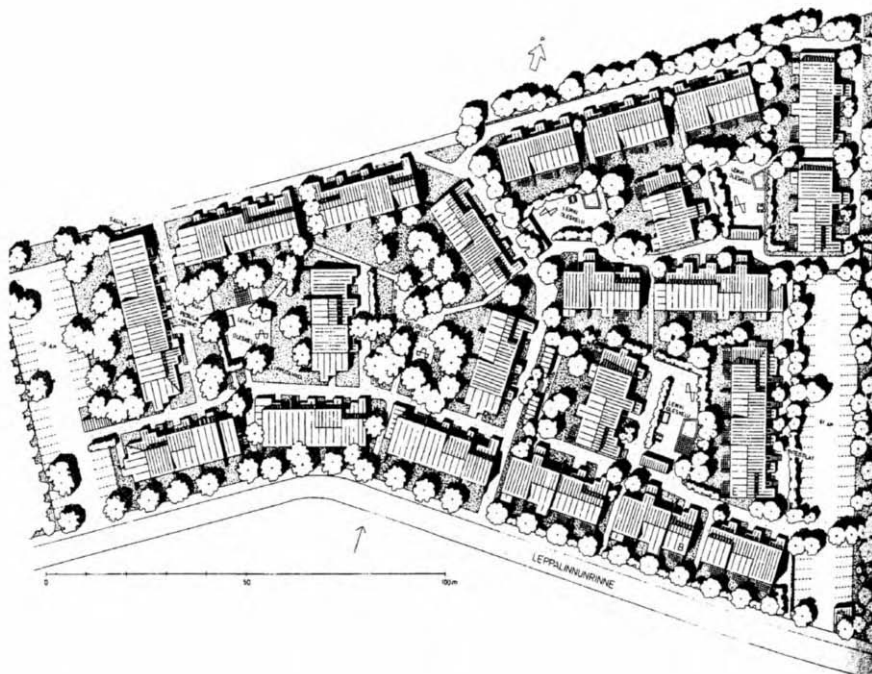
Figure 11. Plan of social housing estate in Leppävaara, revealing a traditional Finnish urban model with small houses round planted courtyards (Hall 1991)
